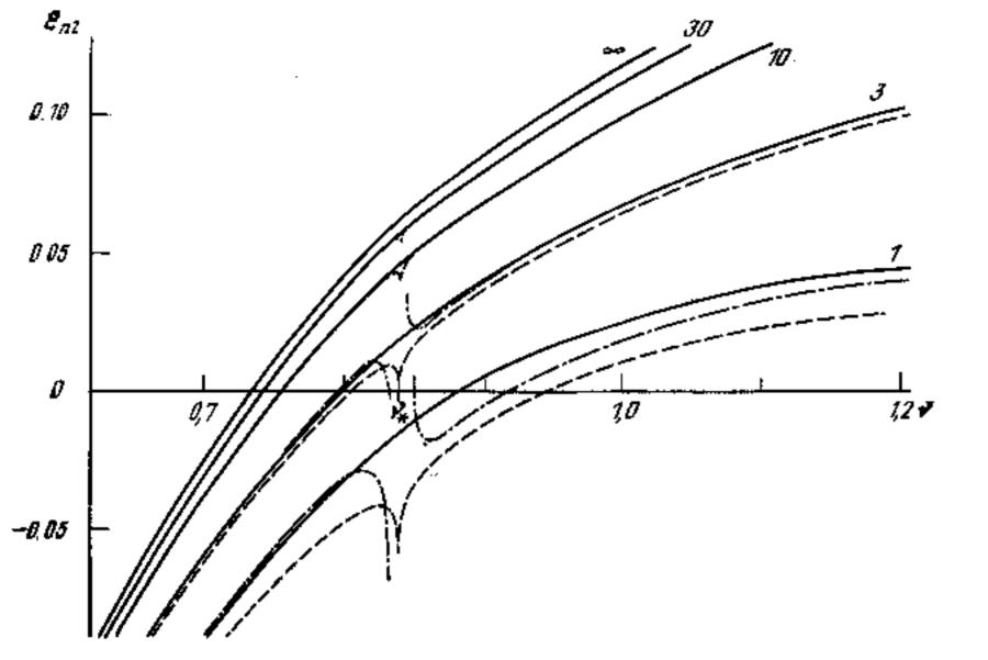
FIG. 1. Energies of the states with l = n - 1 in the Yukawa potential [for  $v > (v_{cr})_{nl}$  we show Re  $\varepsilon_{nt}$ ]. The solid, dashed and dash-dot curves correspond to one, two, and three terms of the series (2.3). The curves are labeled by the / values.
