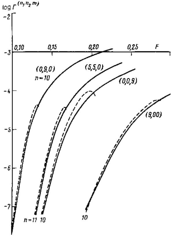
FIG. 1. Width of the levels in a hydrogen the versus reduced field  $(\hbar = e = m_e = 1)$ . The curves are labeled with the parabolic quantum numbers  $n_{\rm D}$  $n_0$ , m and also with the value of n.
